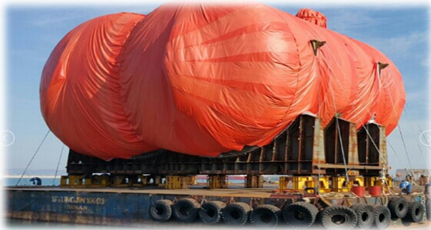
Semi – Pressurized Type 22K LPG Gas Carrier Tank
