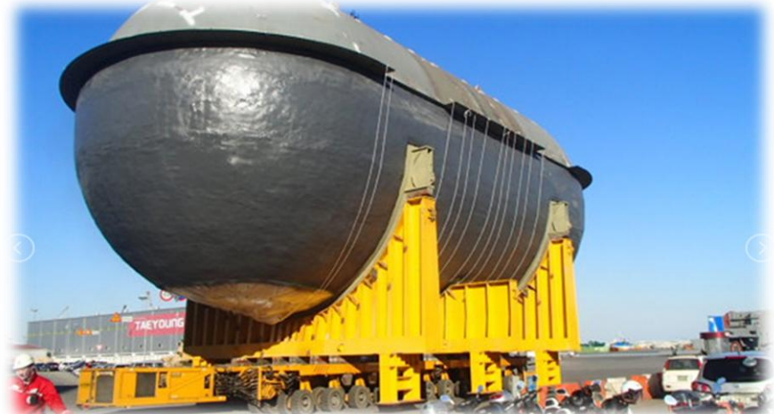
Fully – Pressurized Type 5K LPG Gas Carrier Tank
