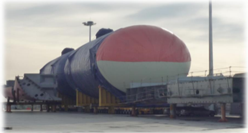
Semi – Pressurized Type 9K LPG Gas Carrier Tank.
