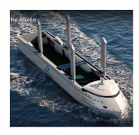
Canopee, the first modern wind powered ship dedicated to Ariane 6 transport. 120m long ship equipped with 4 Oceanwings
