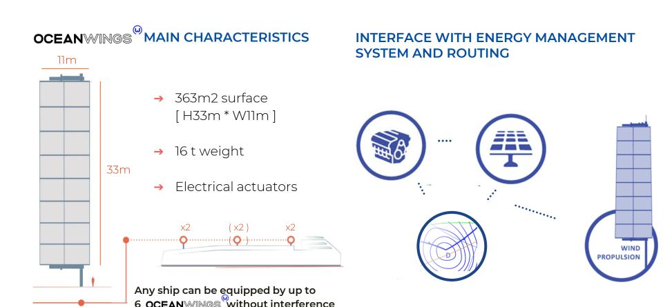
The easiest wingsail system to install aboard a ship, comparable to a handling crane setup...
